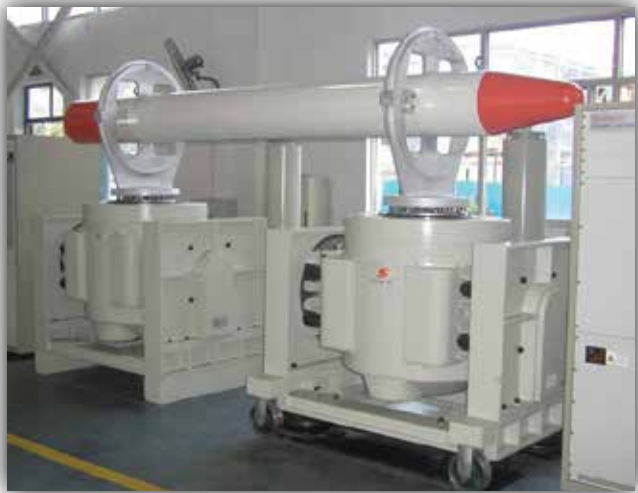
Dual Shaker Vertical Push-Push Arrangement
